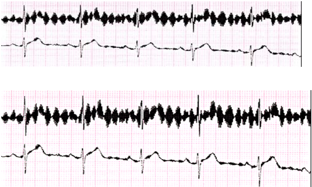
Figure (16) Sixty Hz electrical interference
