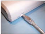
Connect the Type B plug to the rear of the Electronics Module
