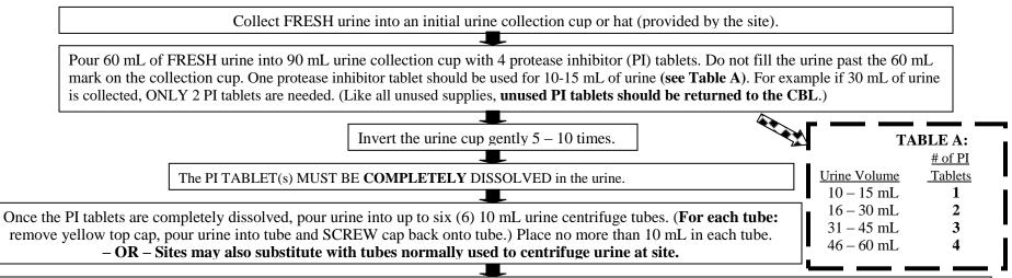
Centrifuge urine tube(s) at MAX SPEED between 1100-1300g (3000rpm with 10cm radius rotor) for 10 mins (swinghead units) **OR** 15 mins (fixed angle units).
