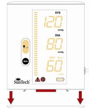
3. Slide the pulse oximetry module along the guides on the bottom of the main BP module from front to back until it snaps into place. All the segments of the pulse oximetry module display will light when the modules have been connected correctly.
